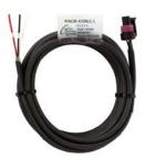
The cable is available in either 20', 40 or 60' lengths with a removable Packard connector to provide easy serviceability. The wire is sealed and crimped to the Packard connector providing a liquid tight environment and strain relief. Media compatibility: Refrigerants (freons) and ammonia.
